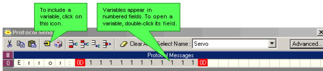
The PLC sends messages via the Configuration linked to the Send operation. These are the types of variables that can be attached to an outgoing message.
