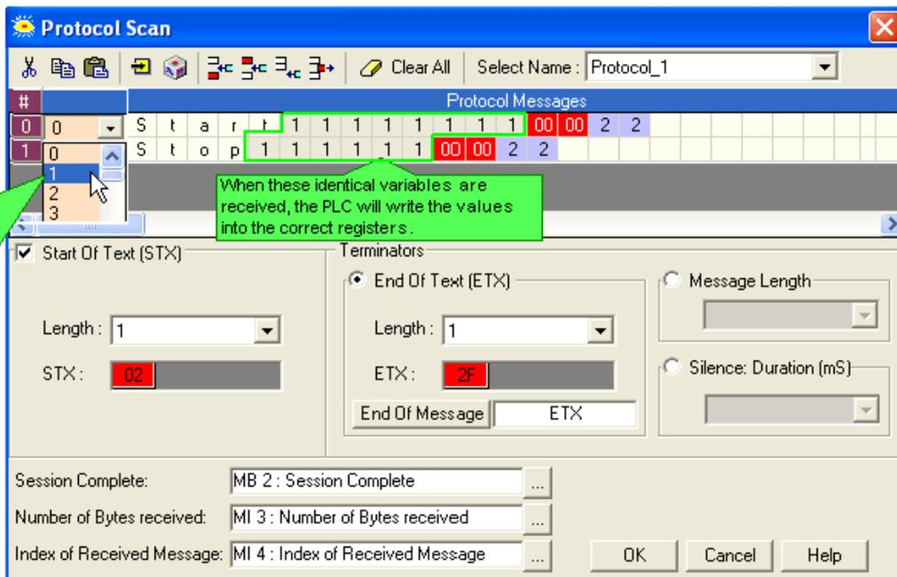
When these identical variables are received, the PLC will write the values into the correct registers.
