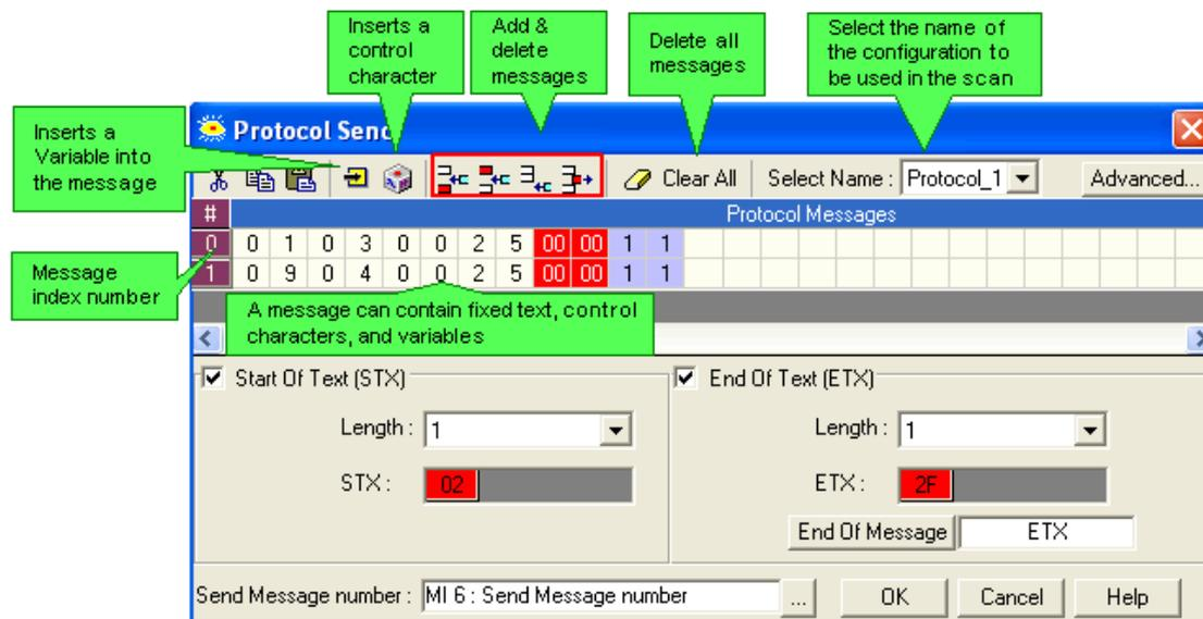
Start of Text (STX)      Check Start Of Text to use an STX parameter to indicate the beginning of a message.
