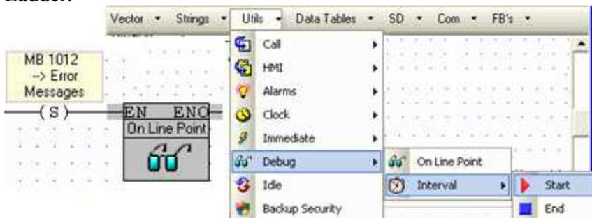
When the scan reaches an OnLine test point that is active (receives RLO), Online Test freezes, enabling you to check element status and values, including Timer values, at that point during Ladder execution. Note that if more than one OnLine test point is activated, SB 35 turns ON.
